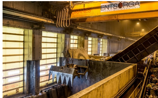
(4) AUTOMATIC BRIDGE CRANE SPIDER™ FOR THE MATERIAL MOVING
